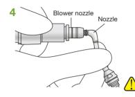
Use the blower nozzle in the same way to clear the lines in the smartGun PERIO nozzle. Blow from the far end of the nozzle.
