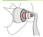
Replace the O-ring(s) at the handpiece joint section of the powder case, apply a drop of the supplied turbine oil and rub it in with your finaers.
