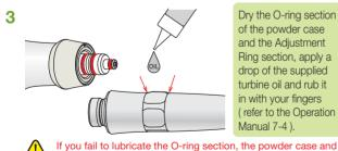
Dry the O-ring section of the powder case and the Adjustment Ring section, apply a drop of the supplied turbine oil and rub it in with your fingers ( refer to the Operation Manual 7-4).
