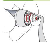
Replace the O-ring(s) at the handpiece joint section of the powder case, apply a drop of the enclosed turbine oil and rub it in with your fingers.
