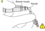
Use the blower nozzle in the same way to clear the lines in the smartGun ONE nozzle. Blow from the far end of the nozzle.
